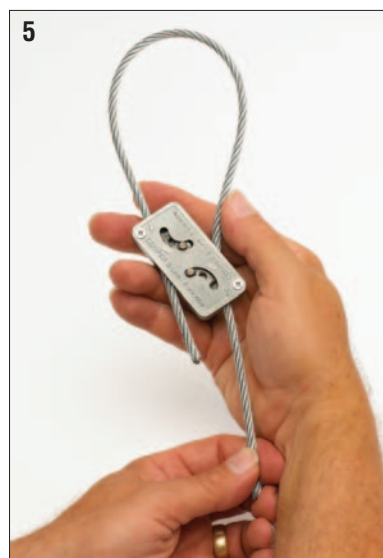
(5) To adjust, remove tension and pull wire rope slightly to disengage teeth, slide adjustment pin in direction shown by arrow to release wire rope.
